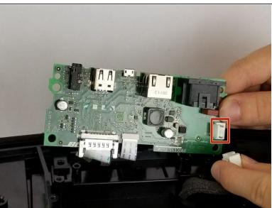
Remove the white cable by pressing on the side of the connector with a tab and pulling backwards.
