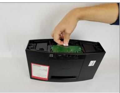
Gently pull the white ribbon from the connector on the top side of the power board.
