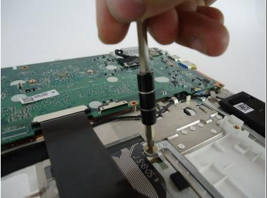
• Remove the (3) three 7.0mm screws using the J0 screwdriver head.
