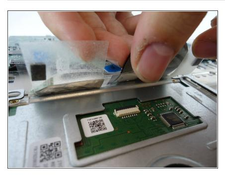
Peel the tape that is on top of the trackpad.
