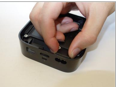
Pull the power port away from the side of the casing.
