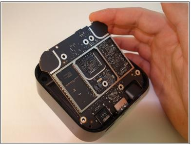
Use the plastic opening tool to tip the board upward.
