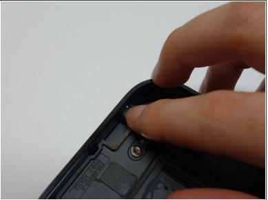
Dislodge the rubber power indicator light cowling's adhesive with a fingernail.
