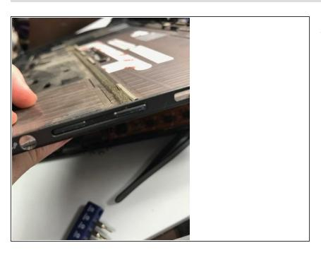
Now that the back panel has been removed, using your fingers, push out the volume button from the inside.
