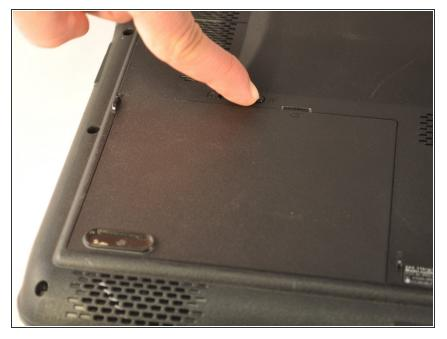
Slide the tab over to unlock the battery cover located on the bottomleft corner of the laptop.
