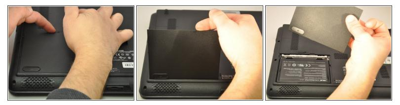
• Lift the exposed lip and remove the battery cover.
