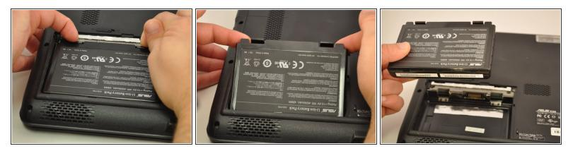
• Press the tabs on the battery and lift them. The battery should come out easily.
