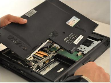
Remove the bottom panel by sliding it toward the hinges and lifting the back panel up.
