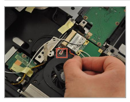
Unplug the wire cable attached to the fan by pulling it out.
