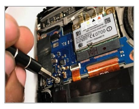
Using the FH000 phillip screwdriver, unscrew the screw that connects the battery to the motherboard, releasing the battery.
