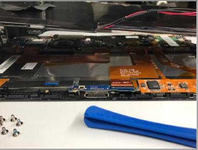
• After all the screws are removed, and all wires are detached, lift the battery away from the tablet.
