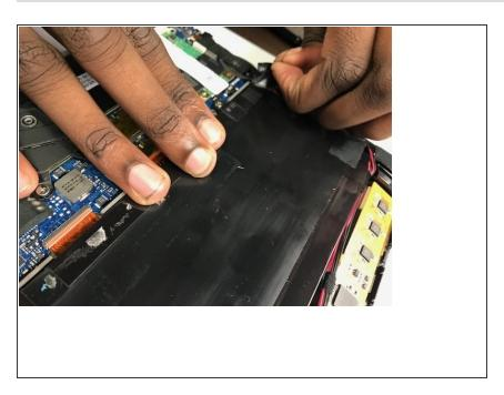
With the back panel removed, take the tape off the battery restricting it from coming loose.
