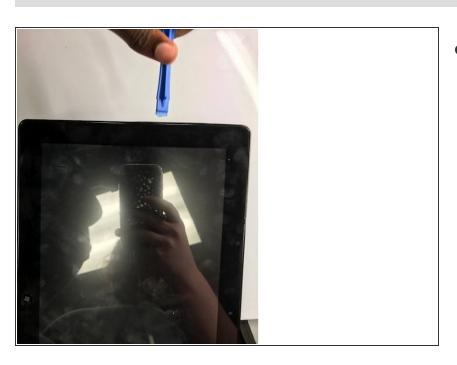
Remove the microSD card before attempting to open the device. Wedge the opening tools inside the device and move it around the perimeter (between the black and silver panels, not between the glass and the black panel) until you have loosened the adhesive that is keeping it together.
