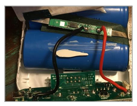
There is a smaller circuit board, presumably for voltage regulation, that connects to the battery bank and then, via red and black wires, to the main circuit board.
