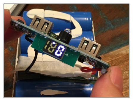
Here's the LED number display. Note that I've briefly pushed the small button on the right side and the display shows zero charge.
