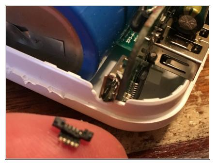
This is why I was unable to charge the iMuto charger... The small fivecontact metal connector (on my finger tip) that is internal to the micro USB port (on the left side of the main circuit board, just above my finger tip) had broken off and fell inside the iMuto charger.
