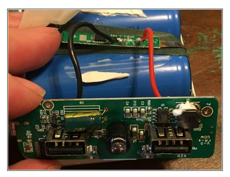
Here's a look at the main circuit board. The micro USB charging port is hidden at left, the two main USB
