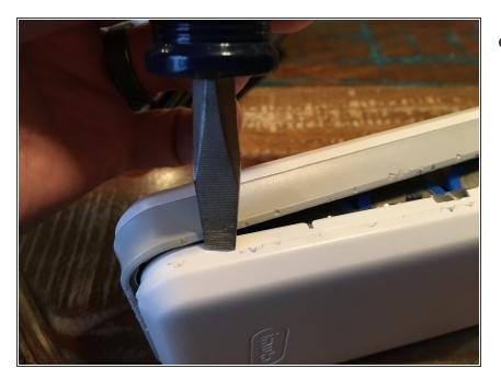
Using a screwdriver, wedge between the plastic band and the case top, then use a twisting motion in the direction like you would driving a screw to work your way around the case, prying the case top from the middle band of plastic.
