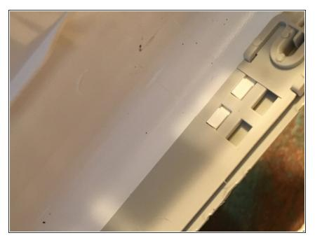
Once you ungracefully chop and pry the case off of the charger, you can see why it is not meant to be disassembled or repaired. The case has clips that hold the case together and these clips can't be easily unclipped.
