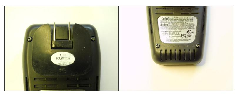
• Use a small screwdriver to remove the four screws on the rear corners of the case.
