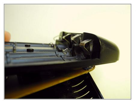
Insert the PCB through the front half of the case, making sure that the LED and battery contacts come out fully on the other side of the case (as seen in photo).
