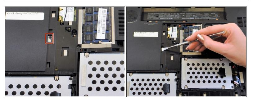
Press the tab with a metal spudger that is located next to the screw to release the optical drive.
