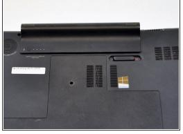
• Slide the battery release latch to the left which is located on the right-hand side of the battery.
