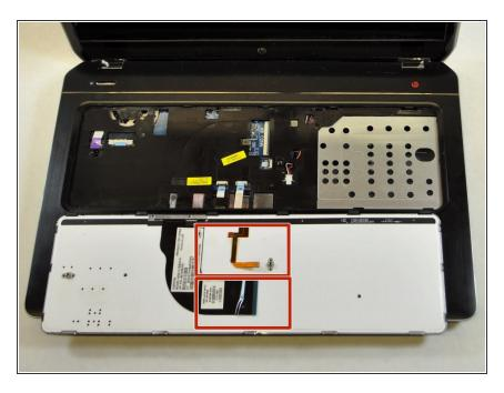
Release the connectors that attach the keyboard to the laptop.
