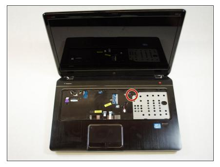
Remove the screw located to the upper left of the disc drive.
