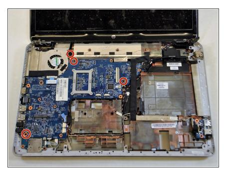
Remove the screws that hold the motherboard to the frame
