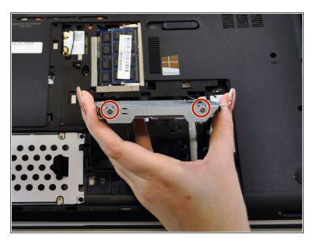
Remove the 2 Phillips PM2.5×5.5 screws on each side of the drive bracket.
