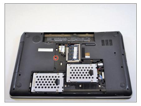
Remove the Phillips PM2.5×4.0 screw that attaches the optical drive to the laptop.
