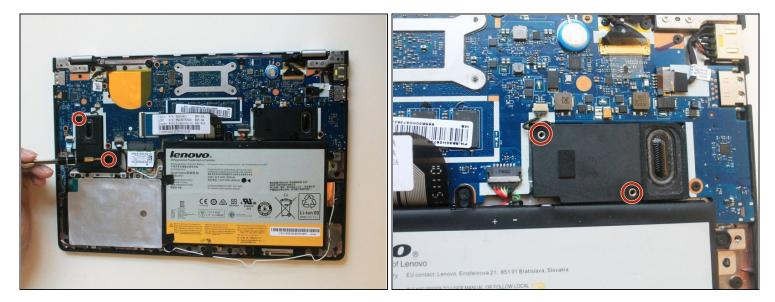
• Remove 2 screws (2mm) from each of the speakers, 4 screws total, using the PH #000 screwdriver.
