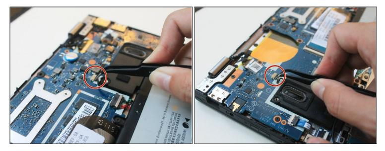
• Unclip the cables by pulling downwards gently using <u>tweezers</u>.
