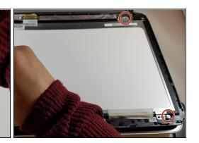
Remove the four 2.86 mm JIS#0 screws from each corner of the silver frame that is holding the digitizer.
