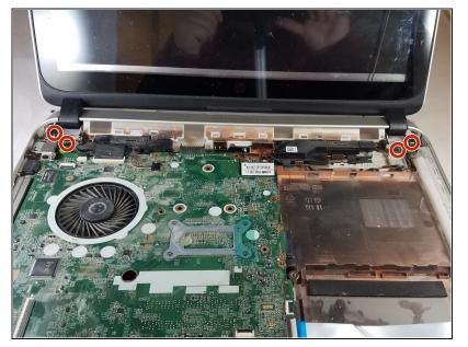
Remove the four 5.66 mm PH#0 from under the keyboard near the hinges.
