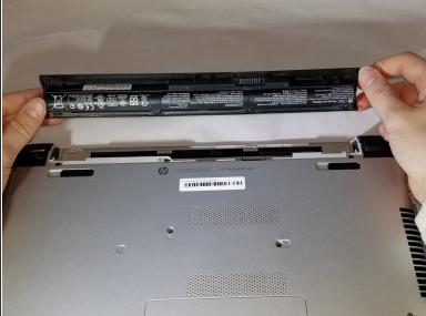
Lift the battery upwards and out from the laptop
