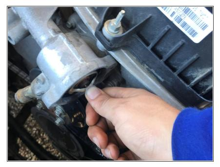
Note that if any antifreeze leaked throughout the process of replacing the thermostat, put more antifreeze in the car after you reassemble everything back to normal.
