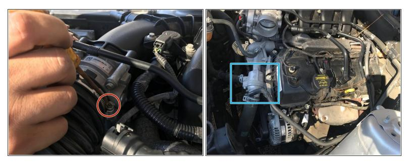
• The second picture is what it should look like once you remove the cold air intake. The thermostat is located by the blue box.
