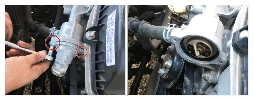
• Remove the housing cover to see the thermostat. The second image shows this.
