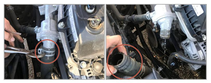
When you remove the hose, make sure and keep it tilted upright so that you don't leak any antifreeze. The second image shows how you should do this.
