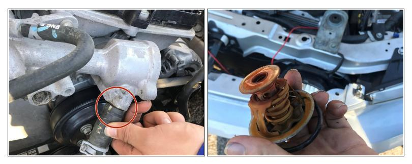
• The second picture shows the old thermostat after being taken out of the housing.
