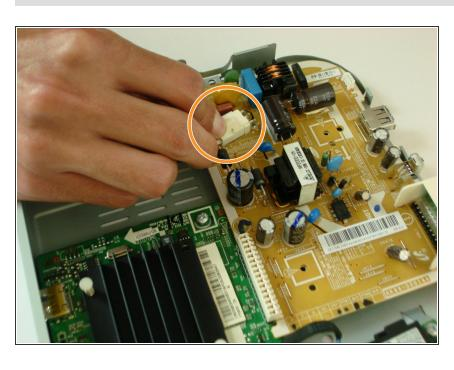
Press down on the plastic retaining clip and pull backwards to remove the AC power connector from the power supply board.
