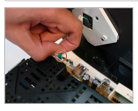
Gently pull up on the ribbon cable by the blue tab to remove it from the power supply board.
