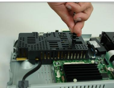
Using a #1 Phillips head screwdriver, remove the two 7.5mm screws on top of the plastic cover and remove the cover.
