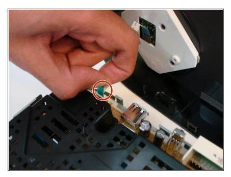
Gently pull up on the ribbon cable by the blue tab to remove it from the power supply board.
