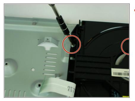
Using a #1 Phillips head screwdriver, remove the two 7.5 mm screws (one not shown) near the front that secures the disc tray to the chassis.
