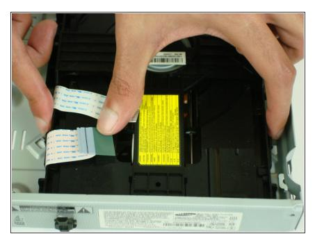
Push two small prongs on either side of disc tray inwards and push disc tray forward.
