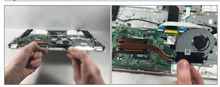
• Using the flat side of the spudger, firmly pry the fan off of the components, as well as the heatsink from the motherboard.
