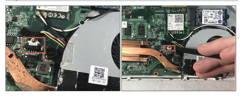
Using the spudger tool, carefully remove the wires connecting the fan to the motherboard.
