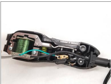
Remove one 7.5 mm JIS #1 screw from the switch base.
