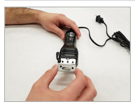
Lift the bottom blade straight up from the device body to remove it.
