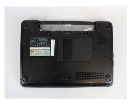
The battery is now fully removed and the laptop will not power on without it.
