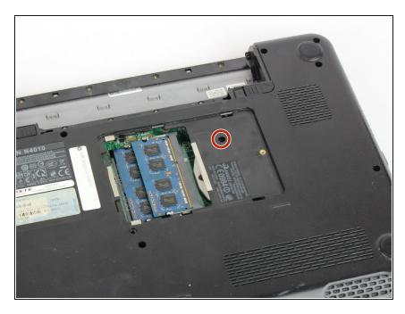
Unscrew the indicated 5.7mm screw beneath the RAM Cover.
