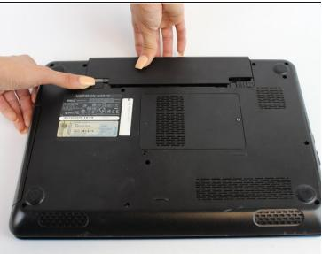
• While holding the left-hand switch to the left position, pull the battery away from the laptop.
