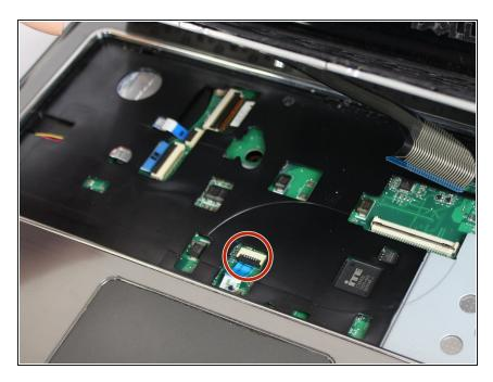
Disconnect the indicated ribbon cables underneath where the keyboard sits.
