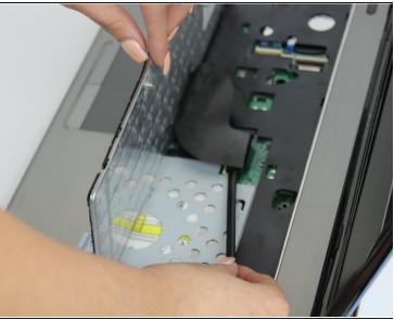
Carefully tip the keyboard upwards and pull it slightly away from the body of the laptop.
