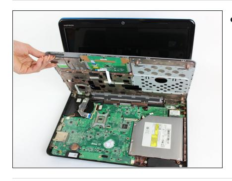
Lift the cover upwards and away from the body of the laptop, after removing the optical drive and unscrewing the three screws on the right
