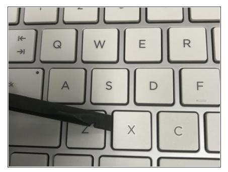
Use a screwdriver or other flat instrument to get under the key, and pull up slightly on one of the edges.
