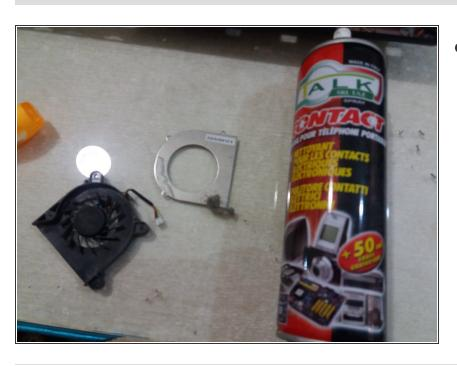
We now clean and remove the dust and sediments that hinder fan function and increase processor heat.
