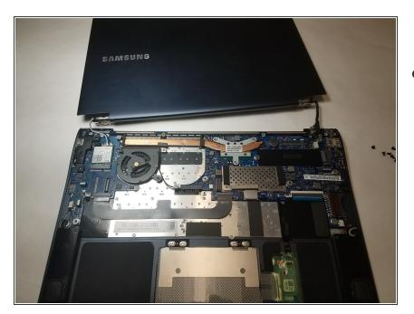
Now the screen is completely disconnected and can just be lifted off.
