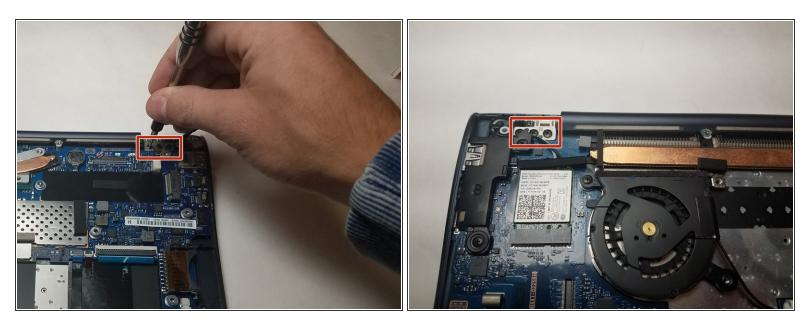
Unscrew the three 4.3 mm screws by using a #000 screwdriver located on the hinges in both corners of the laptop.
