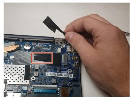
Disconnect the wire connected at the marked location. This is done by giving it a solid tug parallel with the laptop.
