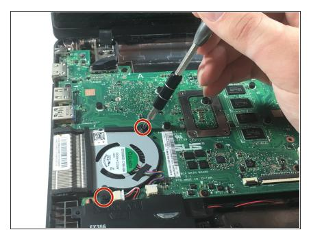
Now, use the Phillips 1 screwdriver to unfasten the two screws holding the fan in place.
