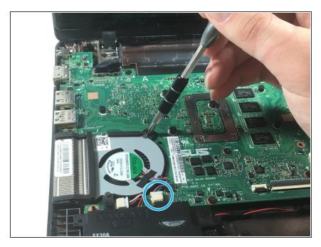
Disconnect the fan by gently pulling the connectors on the wire apart from each other.
