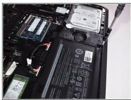
Unscrew the 5 x 2mm x 5mm screws, using the T8 Torx screwdriver.
