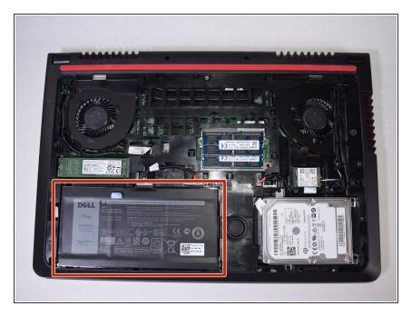
Locate the battery on the bottom left side of the laptop.
