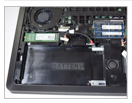
Now lift the battery from the device to remove it.
