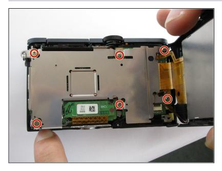
Lift up the screen, and use a Phillips #000 screwdriver to remove the (6) six screws holding down the underlying metal plate.
