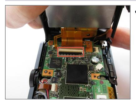
Pull back the black switch holding the orange screen ribbon in place, and remove the screen.
