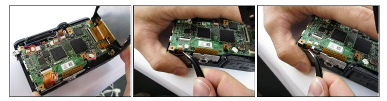
• Using <u>tweezers</u>, pull out the shown connectors
