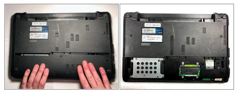
• Slide the back panel off by placing a hand on each corner and pulling the panel towards you.
