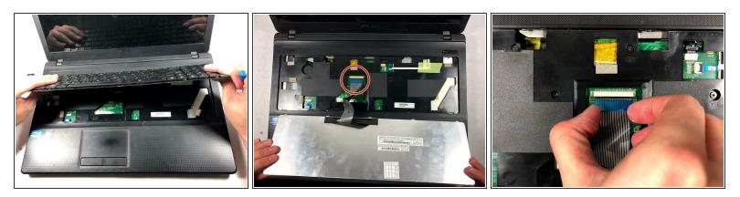
Once the keyboard is free, disconnect the ribbon cable from the zero insertion force (ZIF) connector by flipping up the locking flap and pulling the cable out.
