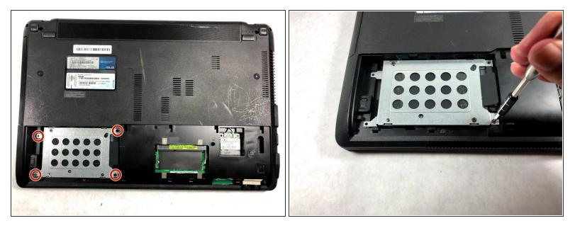
• Remove the four 9mm screws holding the hard drive in place.
