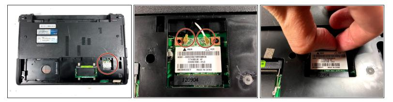
• Disconnect both the black and white coaxial connectors from the WiFi card by pulling up on the gold colored piece.
