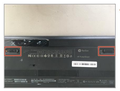
Slide the left release tab toward the center of the computer to the unlock position. Next slid the right tab toward the center of the computer and hold it there while completing step 4.
