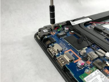
Unscrew the two 1.2 mm screws holding the motherboard to the front panel using the same screwdriver.
