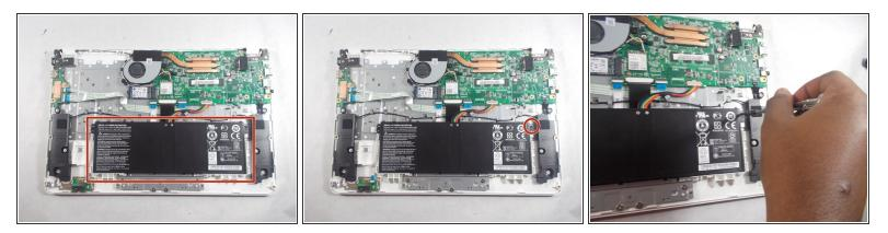
(i) The battery is the large black rectangle located in the bottom center of the device.
