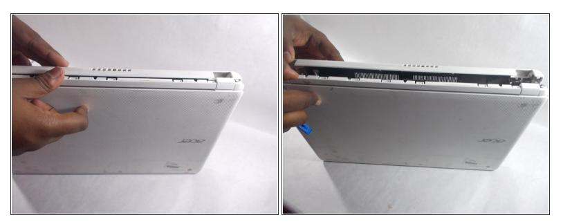
• Stand the device up with the hinges on top and carefully pull apart the back cover from the device.
