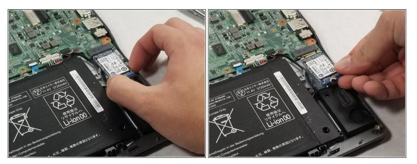
Slide the SSD out of its slot in the motherboard.
