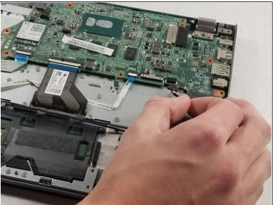
Remove the speaker cable from the motherboard.
