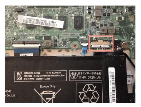
Remove the battery cable attached to the motherboard.
