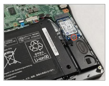
Remove the 5mm screw holding the SSD in place using the Phillips #0 screwdriver.
