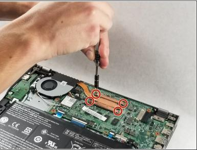
• Remove the four 5mm screws on the heatsink using the Phillips #0 screwdriver.
