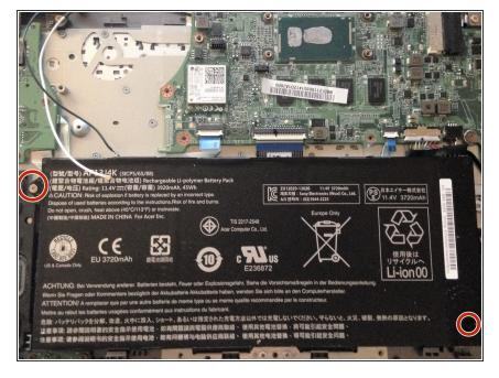
Remove the two 5mm screws holding the battery in place using a Phillips #0 screwdriver.
