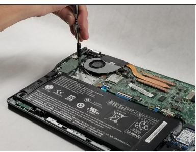
Loosen the two Phillips-head screws on the fan attached to the heatsink.
