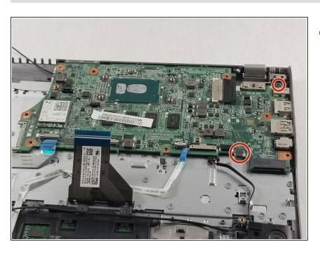
Remove the two 5mm screws holding the motherboard in place using a Phillips #0 screwdriver.
