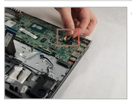
Remove the LCD cable from the motherboard.
