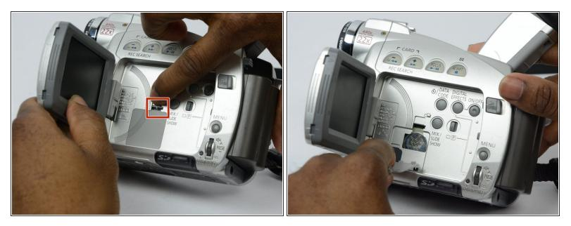
• Open the LCD battery compartment by pulling on the tab as seen in the picture.
