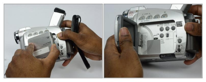
• Open the LCD screen to expose the compartment where the LCD battery is held.
