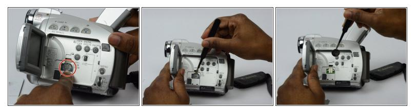
• Use tweezers to carefully pull out the LCD battery.
