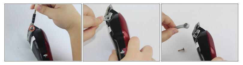
Unscrew the 12 mm Phillip head screw located on the blade adjustment lever using a Phillip's #1 screwdriver. Remove screw from groove to release lever.
