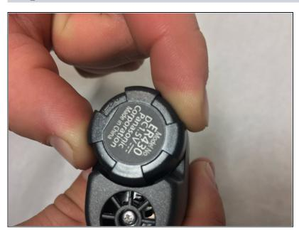
• Twist the battery cover housing in a clockwise direction to secure the the battery.
