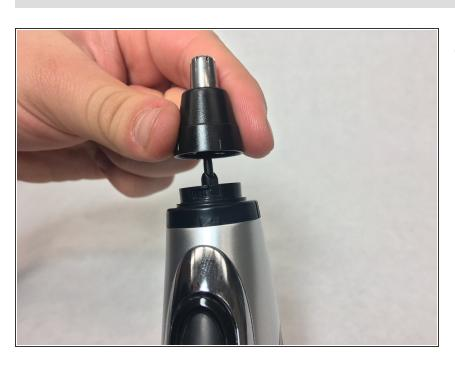
Rotate the blade block counterclockwise and remove.
