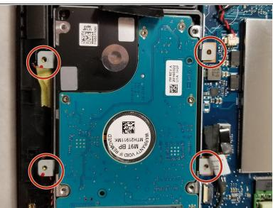
Remove four screws with the Phillips #00 screwdriver.
