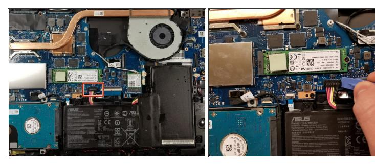
Wedge an opening tool under the battery's bundled cable connector, and gently pry the connector up and to disconnect the battery.
