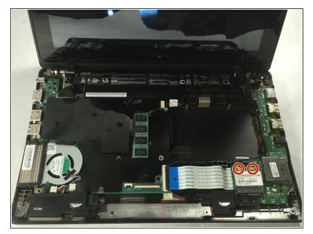
Firstly, disconnect the two tiny wires that connect the audio board to other components. They can be found on a black square near the green decoder strip. Remember to be gentle with these delicate components.
