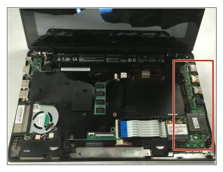
Now, locate the audio board. This model has an L-shaped board. It can be found in the far left region of the internals.
