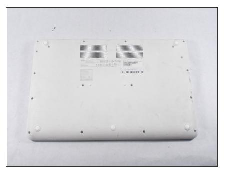
Place the device on a flat surface faced down so that the fan vents are at the top of the device.
