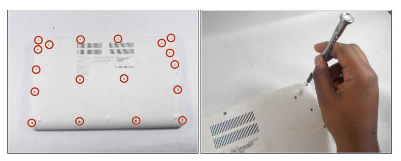
• Unscrew the eighteen 6 mm PH0 Phillips head screws from the back of the device.
