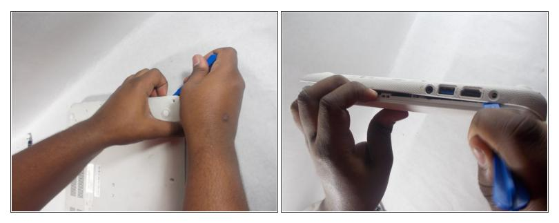
• Use a plastic opening tool to pry open the back cover around the edges of the device.
