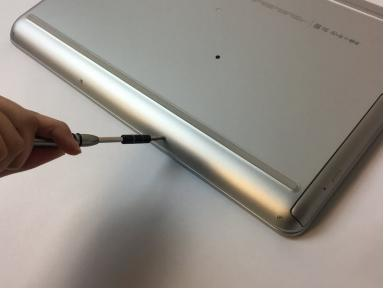
Using a PH0 screwdriver, unscrew the ten 4.4mm Phillips head screws located on the back panel.
