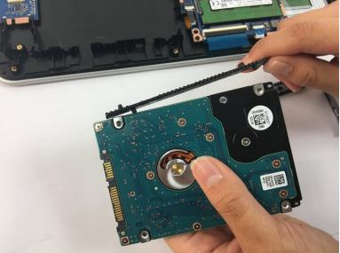
Pull off the plastic wedges on both sides of the hard drive.
