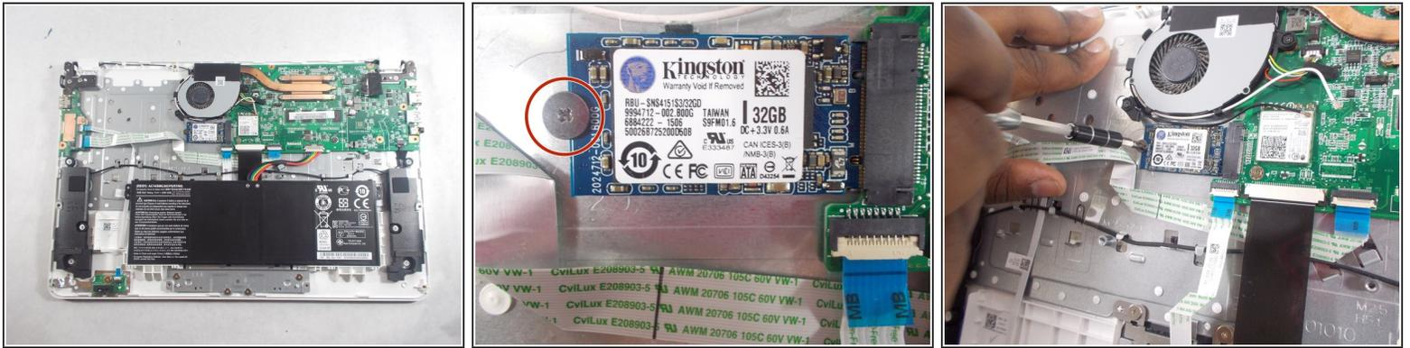
**i** The Solid State Drive is the blue chip locate right beneath the fan.
