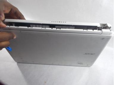
Stand the device up with the hinges on top and carefully pull apart the back cover from the device.
