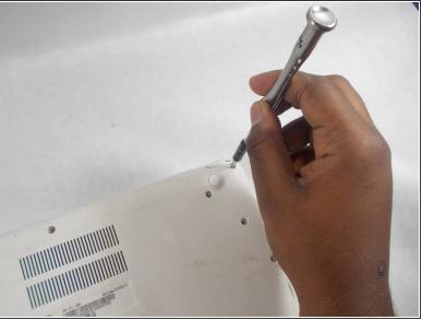
Unscrew the eighteen 6 mm PH0 Phillips head screws from the back of the device.
