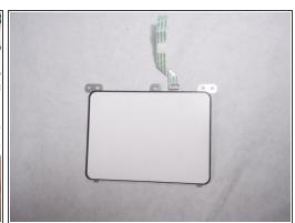
• Grab the track pad from its corners and carefully pull it up and out of the device.
