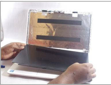
Lift the screen back up from the keyboard and remove from the device.
