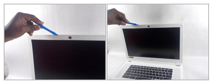
Wedge the plastic opening tool inside the back of the screen cover and run along the perimeter of the screen.
