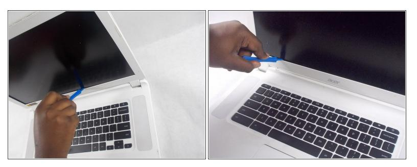
Wedge one of the plastic opening tool in the inside of the screen cover and run it along the inside perimeter of the screen.
