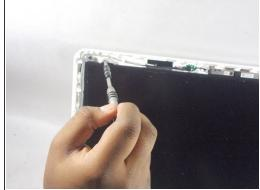
• Unscrew the four 3 mm PH00 Phillips head screws located on the inside corners of the screen.
