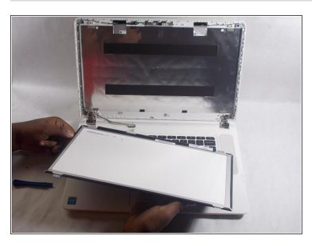
Take out screen from top part of the device and lay it down flat on the key board.
