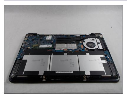
• Locate the battery near the bottom.
