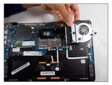
Remove the CPU Fan and Heatsink by simply lifting upwards.
