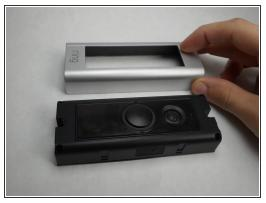
Use your thumbs to apply downward pressure on the glass part of the device while pulling the faceplate up and off of the device.
