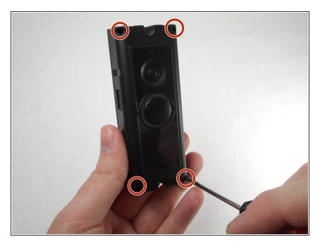
Using a PH-000 screwdriver, unscrew and set aside all four of these 5.25 mm screws.
