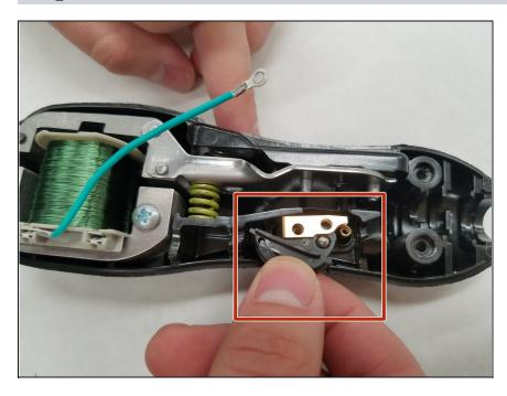
• Remove the switch from device by lifting straight up from the device body.
