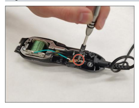
• Remove one 7.5 mm JIS #1 screw connecting the power cord to the switch base.
