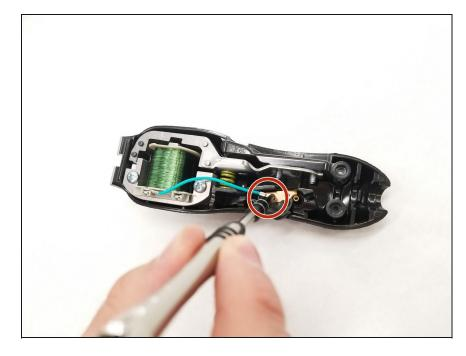
Remove one 7.5 mm JIS #1 screw connecting the wire to the switch base.
