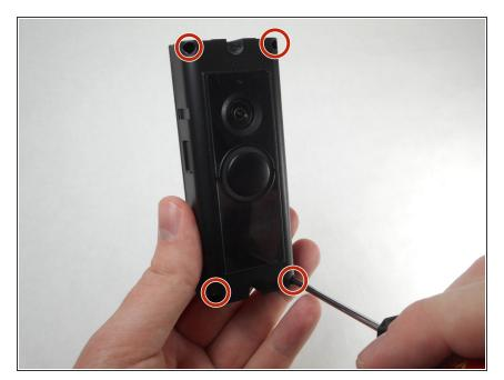
Using a PH-000 screwdriver, unscrew and set aside all four of these 5.25 mm screws.
