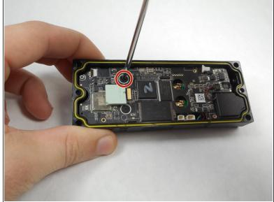
Using the Phillips 000 screwdriver, remove these three 4.25mm screws.
