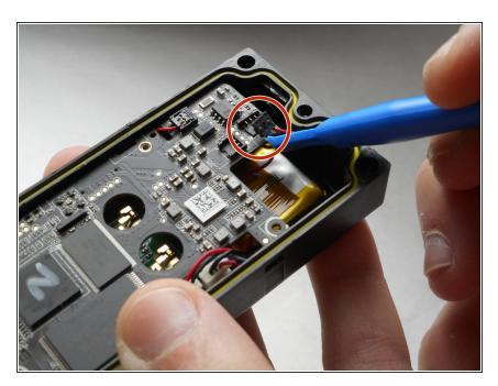
Using the plastic pry tool, carefully remove this wire connection.
