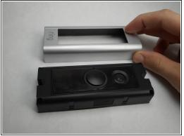
Use your thumbs to apply downward pressure on the glass part of the device while pulling the faceplate up and off of the device.
