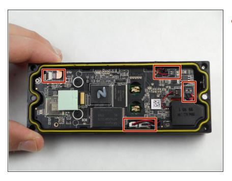
The next step is to remove the last four connections holding the motherboard in place.
