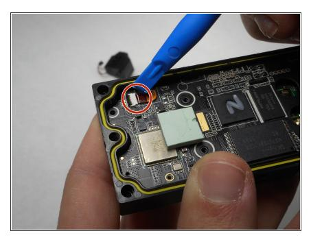
Using the plastic pry tool, gently ease this ribbon cable from its port.
