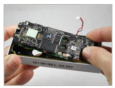
Take the motherboard out of the housing. Lift slowly while doing this to make sure the wires and the delicate ribbon cable are not damaged.
