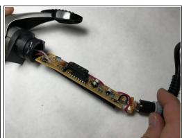
Pry off the housing using a plastic spudger.
