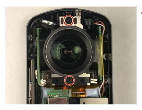
Remove the two 3mm Phillips screws, with the Phillips 00 Screwdriver.
