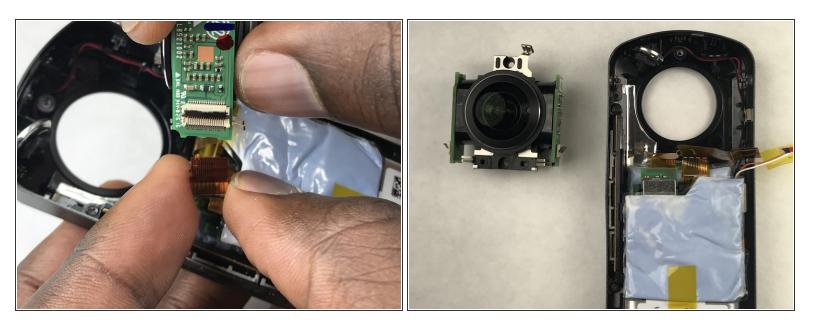
• Carefully detach the two ribbons cables from their connectors to remove the camera assembly.
