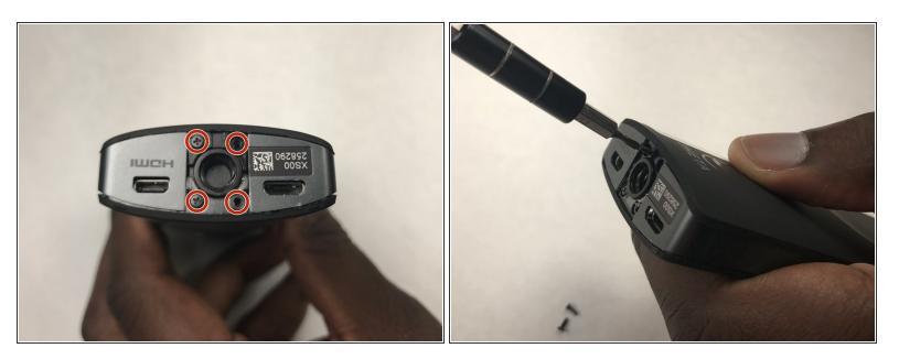
Remove the four 3-mm screws located on the bottom of the device. You will need to use the Phillips 00 screwdriver.
