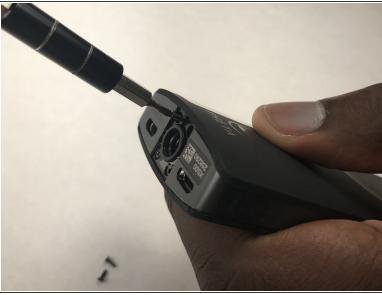
Remove the four 3-mm screws located on the bottom of the device. You will need to use the Phillips 00 screwdriver.
